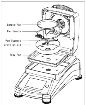
Lift the cover straight up and Install the tray pan in the base of the heating chamber.
