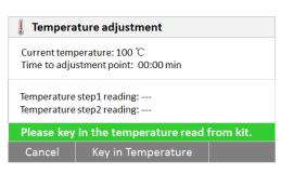
This is a two-point adjustment (100°C and 160°C). The dryer unit now heats to the second temperature (160°C). Adjustment of the temperature is defined by two points. Proceed exactly as you did for the first temperature. After you have set the display to agree with the thermometer, then press the **Enter** button.
