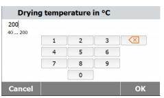
Press the Drying Temperature button to access the temperature setting menu.
