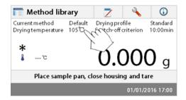
The analyzer comes with a default method preinstalled. The settings of the default method are shown on the display. To edit the settings, press on the area where the settings are displayed as shown to the left.
