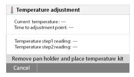
You are now prompted to remove the pan support. Place a temperature calibration kit and close the upper housing.
